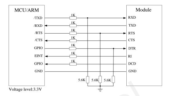
Figure 23: 3.3V level match circuit
