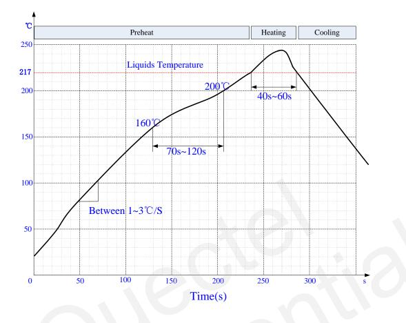
Figure 46: Ramp-Soak-Spike reflow profile
