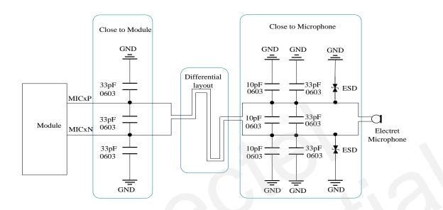
Figure 26: Microphone interface design of AIN1&AIN2
