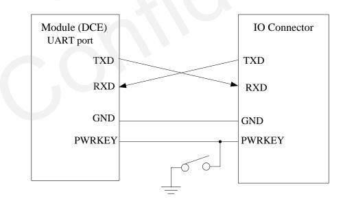
Figure 21: Connection of firmware upgrade
