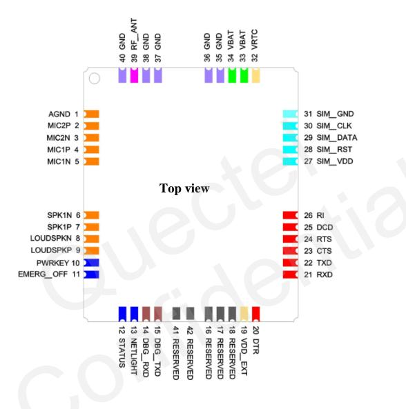
Figure 2: Pin assignment
