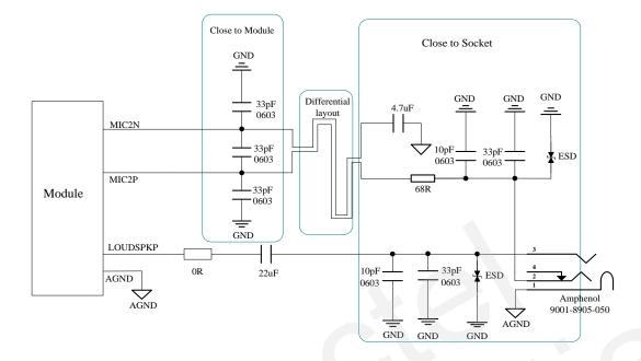
Figure 28: Earphone interface design
