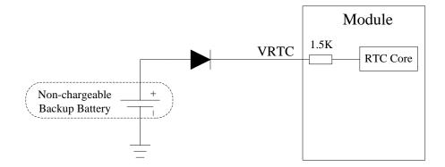
Figure 14: RTC supply from non-chargeable battery
