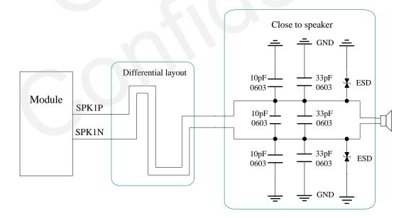
Figure 27: Receiver interface design of AOUT1
