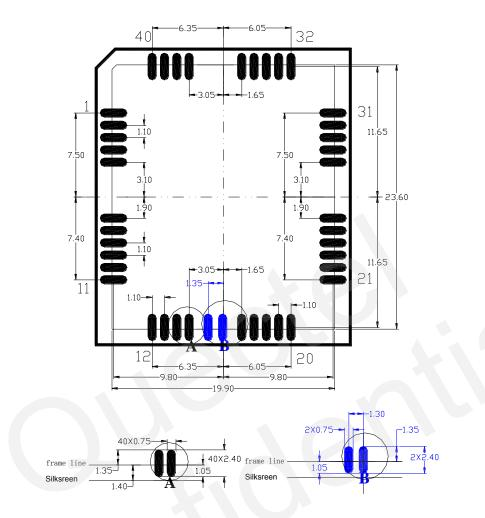
Figure 42: Footprint of recommendation (Unit: mm)
