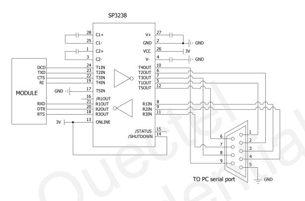
Figure 25: RS232 level match circuit
