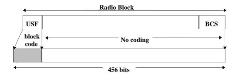
Figure 51: Radio block structure of CS-4
