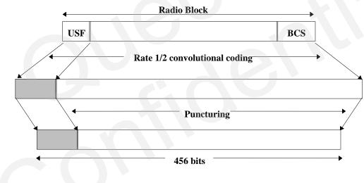
Figure 50: Radio block structure of CS-1, CS-2 and CS-3
