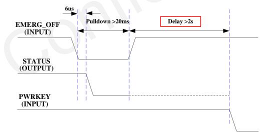
Figure 13: Timing of restarting system after emergency shutdown
